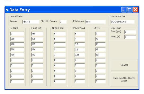
All the parameters are to be fed in desired units to the program, the program then decides the limits for all parameters and suggests suitable grid spacing values, which can be modified by the user. The program adjusts the scale to fit the graphs in A4 size paper sheet. The program then draws the required curves in AutoCAD. The curves can be saved as drawing file in AutoCAD and can be modified there if needed.
