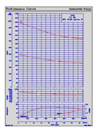
For submersible pumps head curves of different stages can be generated for a model by specifying head values for single stage pump and number of stages for various head curves.
